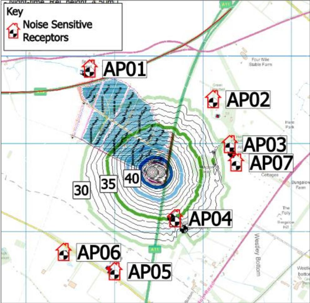
Figure 7: Indicative Night-time Noise Contour Plot, dB LAeq
